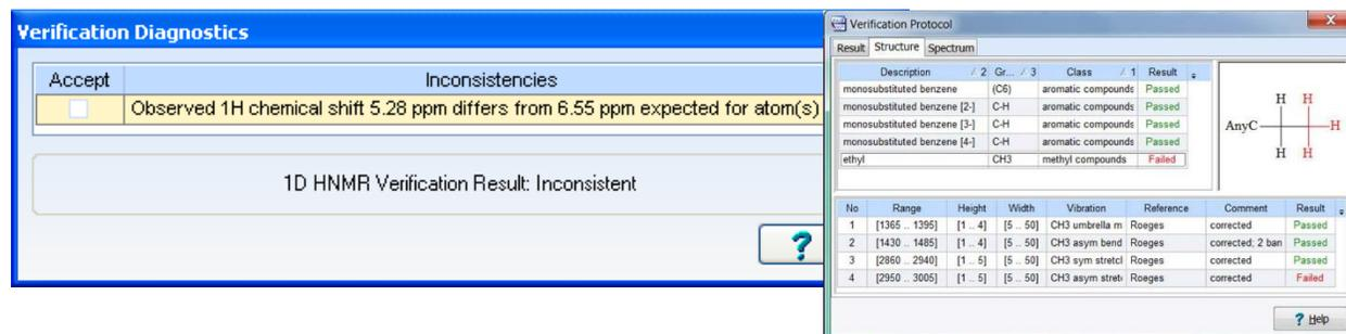
**Figure 8:** Verification output—(left) for NMR, Spectrus Processor provides information about the experimental chemical shift that significantly differs from the predicted for atom 5 in the chemical structure; (right) in the IR protocol inconsistencies between expected spectral bands and structural fragments are flagged for closer inspection.
