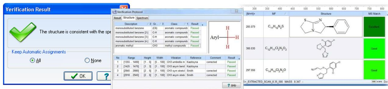
**Figure 7:** Verification output supports faster, more confident decision-making. Left to right:  $^1\text{H}$  NMR—a simple statement that the structure is (or is not) consistent with the spectrum; IR verification—pass/fail for correlation of fragments with bands in the spectrum; MS Match provides a binary result based on the presence of a monoisotopic mass and expected isotopic pattern.
