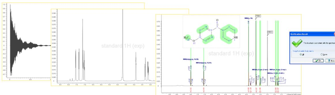
**Figure 2a:** How do you like your data? From left to right: raw NMR data (Bruker FID), processed data (Bruker 1r), fully verified data (ACD/Labs \*.spectrus and \*.esp).
