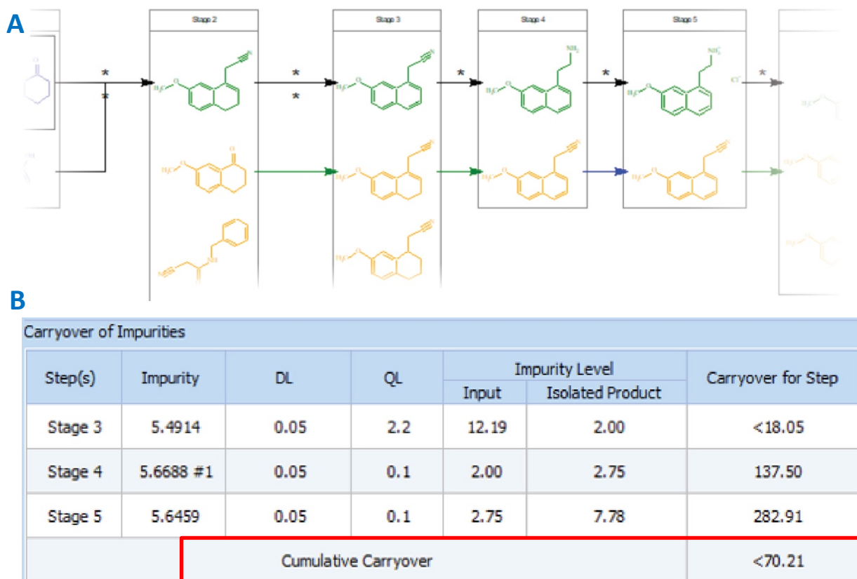
Figure 3 As the reaction pathway for Sulphabenzamide is defined in the Process Map in Luminata (A), the Carryover of Impurities Table (B) populates dynamically where 'DL' and 'QL' represent detection limit and quantitation limit respectively.
