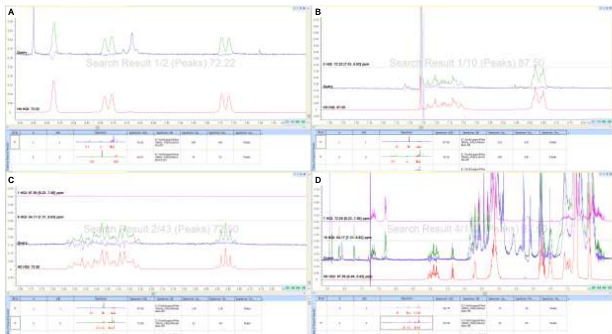
Figure 2. The sequential workflow for component identification from a sample containing an unknown lubricant/alkoxyate mixture by ^1\text{H} NMR Spectroscopy and NMR Workbook Suite. (A) Search was first performed on the 7.53–8.62 ppm region that contains resolved signals. The “Hit Spectrum” (red) is displayed below the query (green) that has the residual curve (purple) overlaid (display can be on or off) and can be adjusted (chemical shift, intensity, line broadening) in order to effectively minimize the residual curve. Once the analysis is satisfied with the search result, the component is selected in the Table of Search Results and a new region can be searched. (B) The search results of the second spectral region (6.23–7.56 ppm) with the second component identified and residual minimized. Upon searching the second region, the first component selected in Table of Search Results is displayed above the query for the analyst’s reference. (C) The search results for the third query region (4.49–5.82 ppm) displaying the identified component and the minimized residual curve. (D) The same result as in (C) zoomed out to highlight that the component fits with the entire query spectrum and that “extra” peaks are not present which would be easily observed by deviations in the residual curve.
