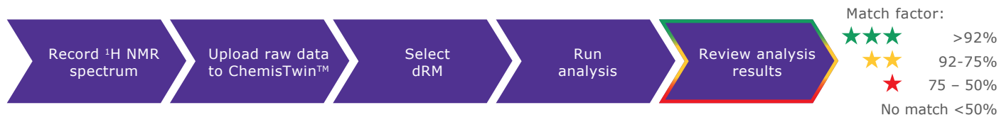
Figure 1. Workflow of the structure verification using ChemisTwin.
