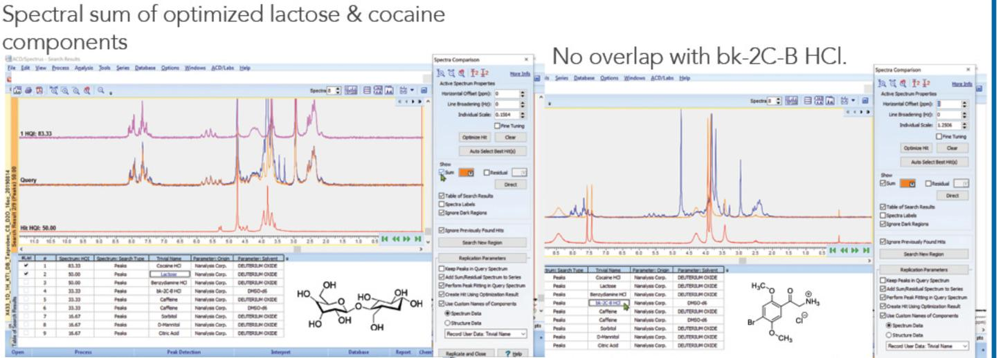
Once complete, one can see the sum of the matching components on the query and get the residual sum of squares, the relative residual and other parameters associated with the match. Additionally, when compared with GC-MS analysis on the same sample, there is excellent agreement.
