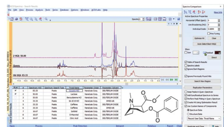
The quality of the fit between the spectra can be visualized using either spectral 'residuals' or'sums'.
