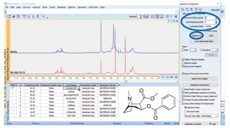
The search returns as a result a number of compounds, in the case of the unknown street drug sample shown here, there are 9 possible hits. The main component is cocaine, with an 83.33 HQI factor, and the remainder of the matches correspond to potential fillers.
