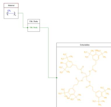
In Figure 3, we can take a material of interest, such as Polypropylene and generate an E&L map. In this case, the extractable would be Irganox 1010. It can also store the degradants that occur for Irganox 1010 as well.
